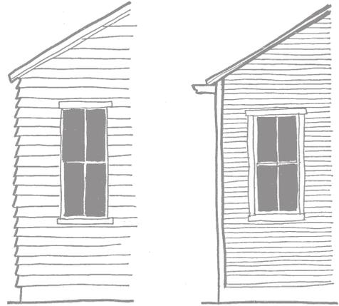
Inappropriate: Wide siding covers corner, sill, and window trim
